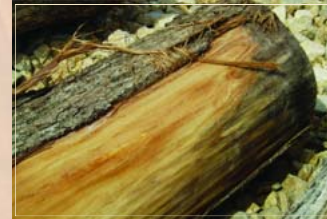
Bark loss on this log during harvesting or transportation provided easy access to fungal spores and subsequent stain development.
