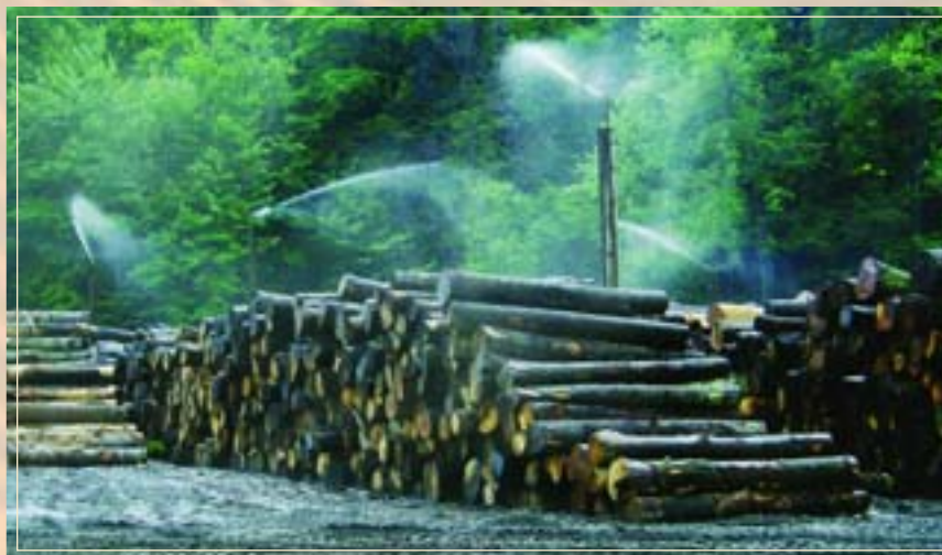
Keeping logs wet can deprive staining fungi of the oxygen they need to grow.
