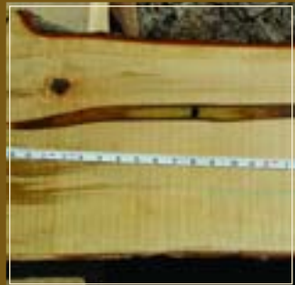
Bore holes from maple taps can provide a convenient entry point for sap-staining fungi to become established.
