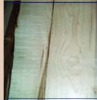
Do not confuse blue stain (top) with heart discoloration (bottom).
