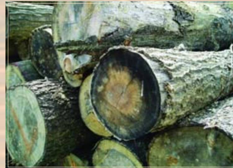
Tight piling and the lack of end coating, water or fungicidal treatment has led to stain development that is sure to spread through this stack.
