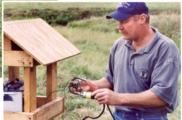
Dick Cates shows the float (above) used to activate a pump submersed in the stream (top photo). The pump is powered with a nearby battery (right) protected from the weather.
